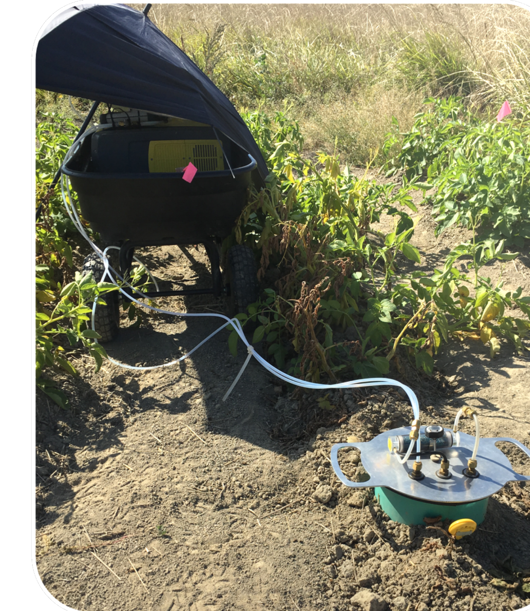
Fig. 3. Gasmeter DX 4040 and static chamber.
